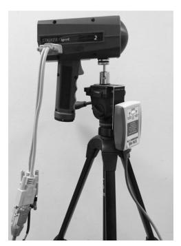
Your scoreboard package includes a radar gun kit. The radar gun can capture the speed of pitches and relay that information to your control console, which sends the data to be displayed on your scoreboard. The radar gun is battery operated and therefore does not require AC power during the game (as long as you keep the battery charged). It communicates wirelessly with the scoreboard control console, so there are no additional cables to run.
